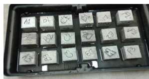
Figure 1 Water absorption test on concrete cubes
